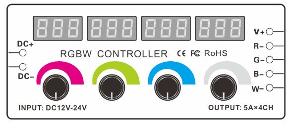
Four rotary knobs to dim Red , Green , Blue and White colors, When rotating the knobs the operation mode shifts to mode I automatically, and the LED digital tube shows the grey scale level of Red , Green , Blue and White under this mode. The LED digital tube indicates current mode, speed and brightness.
